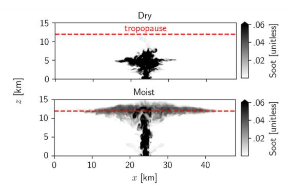
Distribution of soot concentration as a function of height and horizontal distance from the center of the firestorm obtained from large eddy simulations. The dry simulation is on the top, and moist simulation is on the bottom. Soot cross sections are evaluated at the end of simulations and in the center of the domain. The moist simulation uses 70 percent relative humidity. Credit: Tarshish and Romps [2022], Figure 6 (modified)
