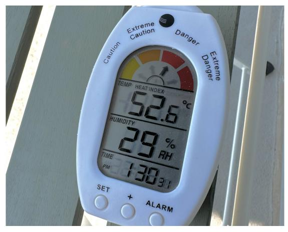
Commercial devices like this are available to calculate the heat index, that is, how hot it actually feels given the humidity. But the algorithm used to compute the heat index breaks down under extreme conditions of temperature and humidity, underestimating the stress on the human body.
